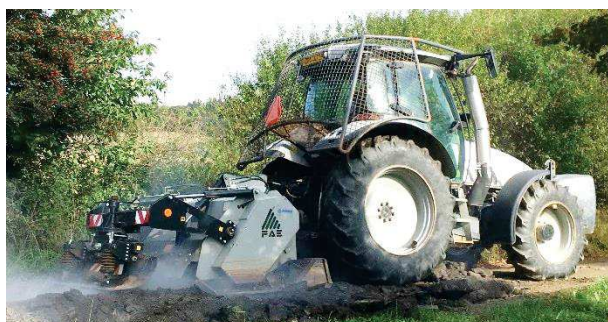
Traktor Lamborghini R6.120 s frézou FAE STC 150
